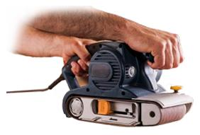
grit or 320-grit paper and moving up to a 600-grit or 800-grit. Use light pressure and keep the sander moving at all times. This will avoid heat buildup and damage to the acrylic. Always wear a mask when sanding to avoid dust inhalation.
